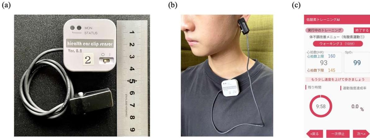
Fig.3. Developed wearable pulse oximeter and dedicated smartphone application. (a) Developed wearable pulse oximeter. (b) Wearing of the developed wearable pulse oximeter. (c) Screenshot of the dedicated smartphone application.
