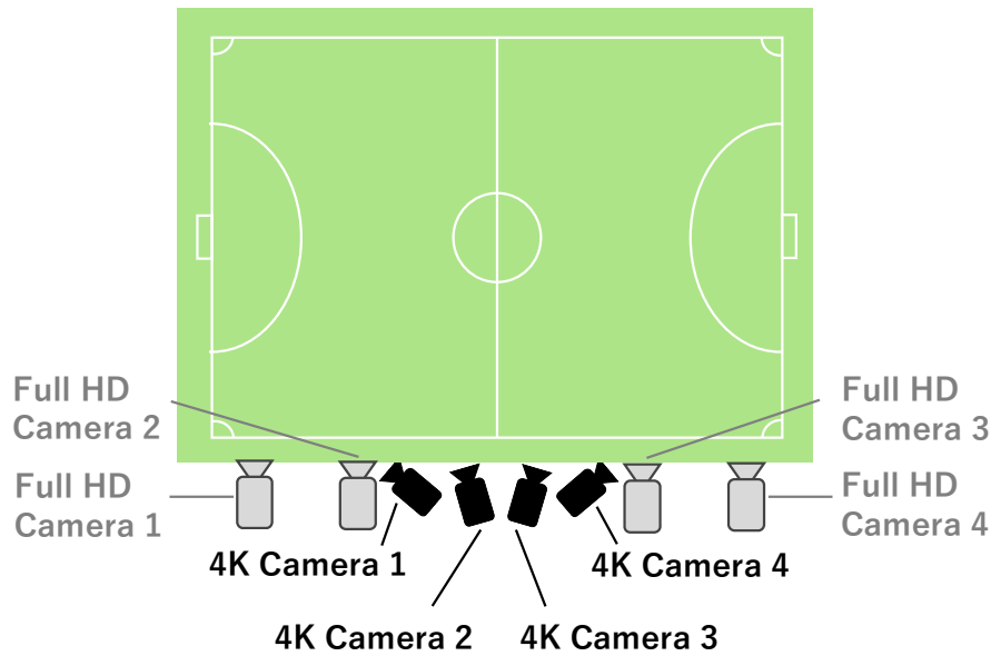
Fig. 6. Position of installing video cameras for futsal
